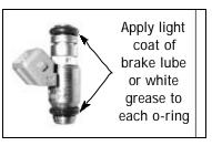
press down until the fuel injectors are seated into the fuel rail. NOTE: It may be helpful to press one injector into the fuel rail at a time. The o-rings will allow enough flex
